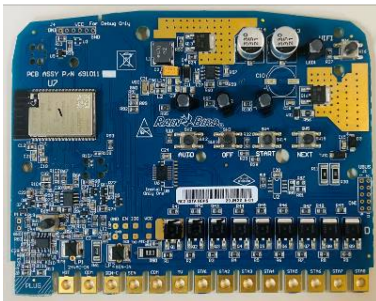
Photo 3: Interior of RC2I8-230 – Control board
